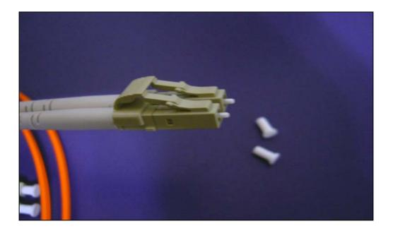
5. Plug the LC/LC Fiber Cable into the transceivers on both Switch.
