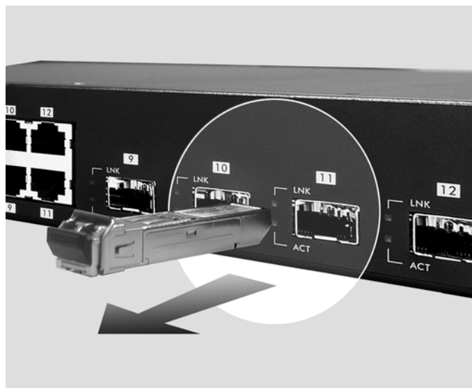
Figure 3-5 Transceiver Removal Example
