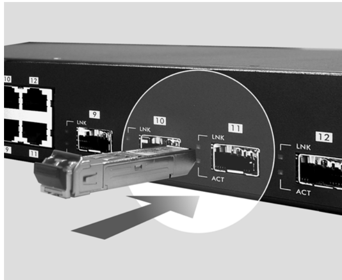
Figure 3-2 Transceiver Installation Example
