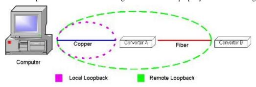
Dip Switch 6 ON: enables local loop back function
