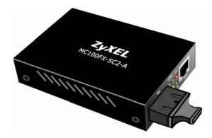
The MC100FX-SC30-A media converter comes with a built-in single-mode fiber transceiver module with SC connector that can be used for distances of up to 30km.
