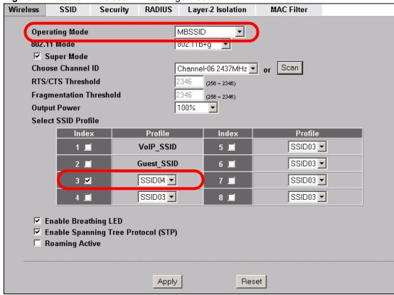
This **Select SSID Profile** table allows you to activate or deactivate SSID profiles. Your wireless network was previously using the **SSID04** profile, so select **SSID04** in one of the **Profile** list boxes (number **3** in this example).
