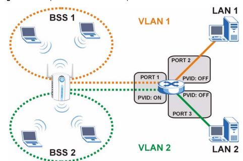
Figure 55 Multiple BSS with VLAN Example
