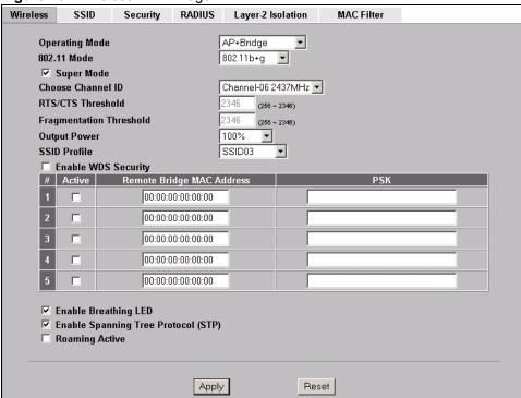
See the tables describing the fields in the **Access Point** and **Bridge/Repeater** operating modes for descriptions of the fields in this screen.
