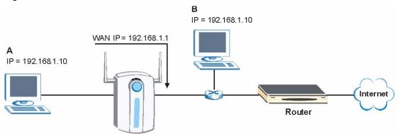
You must set the ZyXEL Device to use different LAN and WAN IP addresses on different subnets if you enable DHCP server on the ZyXEL Device. For example, you set the WAN IP address to 192.59.1.1 and the LAN IP address to 10.59.1.1. Otherwise, It is recommended the ZyXEL Device uses a public WAN IP address.
