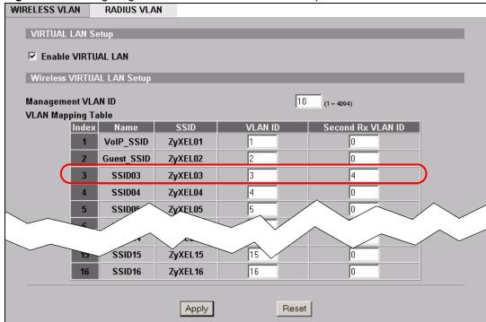
6 Click **Apply** to save these settings. Outgoing packets from clients in **SSID03** are tagged with a **VLAN ID** of **3**, and incoming packets with a **VLAN ID** of **3** or **4** are forwarded to **SSID03**.
