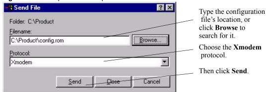
After the configuration upload process has completed, restart the ZyXEL Device by entering "atgo".
