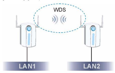
Be careful to avoid bridge loops when you enable bridging in the ZyXEL Device. Bridge loops cause broadcast traffic to circle the network endlessly, resulting in possible throughput degradation and disruption of communications. The following examples show two network topologies that can lead to this problem:
