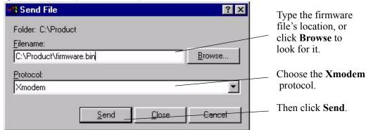
After the firmware upload process has completed, the ZyXEL Device will automatically restart.
