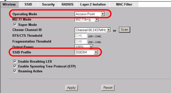
Select **MBSSID** from the **Operating Mode** drop-down list box. The screen displays as follows.
