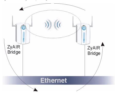
Figure 41 Bridge Loop: Bridge Connected to Wired LAN
