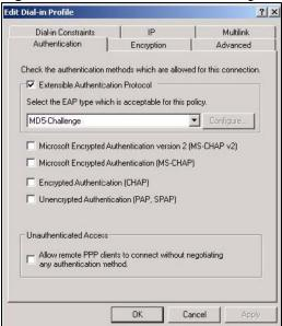
**8** Click the **Encryption** tab. Select the **Strongest** encryption option. This step is not required for EAP-MD5, but is performed as a safeguard.
