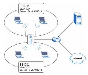
Packets sent from the server S back to the switch are tagged with a VLAN ID (incoming VLAN ID). These incoming VLAN packets are forwarded to the ZyXEL Device. The ZyXEL Device compares the VLAN ID in the packet header with each SSID's configured VLAN ID and second Rx VLAN ID settings.
