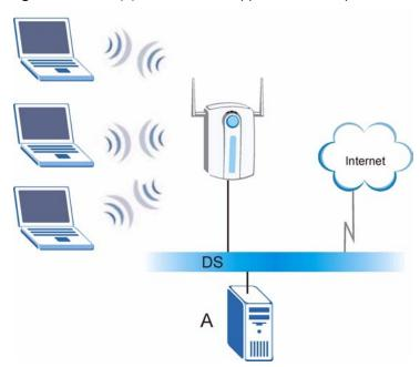
Figure 46 WPA(2) with RADIUS Application Example
