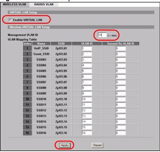
**4** The ZyXEL Device attempts to connect with a VLAN-aware device. You can now access and mange the ZyXEL Device though the Ethernet switch.
