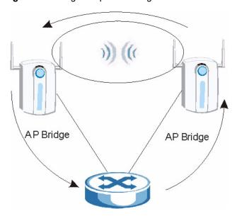
• If your ZyXEL Device (in bridge mode) is connected to a wired LAN while communicating with another wireless bridge that is also connected to the same wired LAN.
