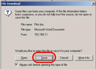
**5** Save the friendly AP list somewhere it can be accessed by all the other access points on the network. In this example, save it on the network file server (**E** in Figure 24 on page 53). The default filename is "Flist".
