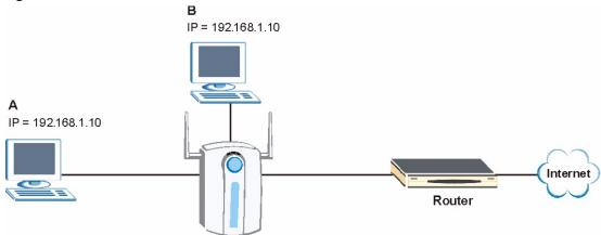
This problem can be solved by adding a VLAN-enabled switch or set the computers to obtain IP addresses dynamically.
