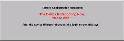
The ZyXEL Device automatically restarts in this time causing a temporary network disconnect. In some operating systems, you may see the following icon on your desktop.
