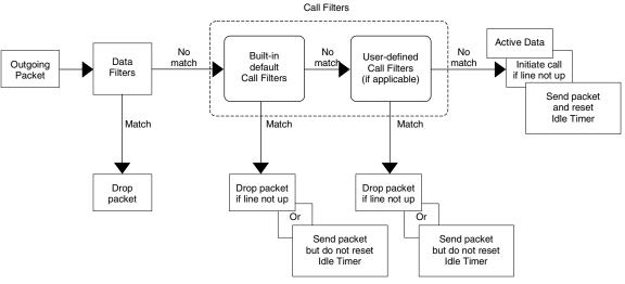
**Figure 9-2 Outgoing Packet Filtering Process**
