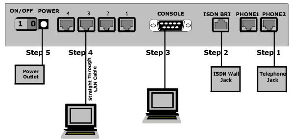
Figure 2-2 Prestige 100IH Rear Panel and Connections
