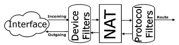
Figure 9-6 Protocol and Device Filter Sets
