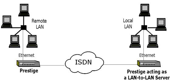
Figure 7-2 Example of a LAN-to-LAN Server Application
