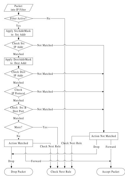
Figure 9-8 Executing an IP Filter
