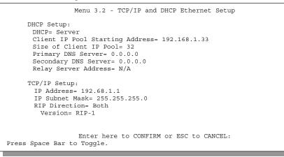
Figure 3-1 Menu 3.2 – TCP/IP and DHCP Ethernet Setup
