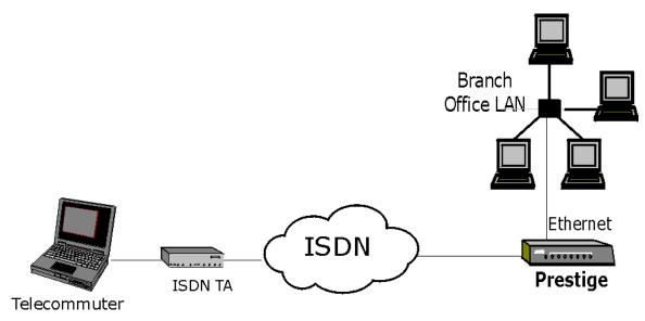
Figure 1-3 Telecommuting/Remote Access Server Application
