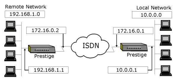
Figure 6-3 Sample IP Addresses for a TCPI/IP LAN-to-LAN Connection
