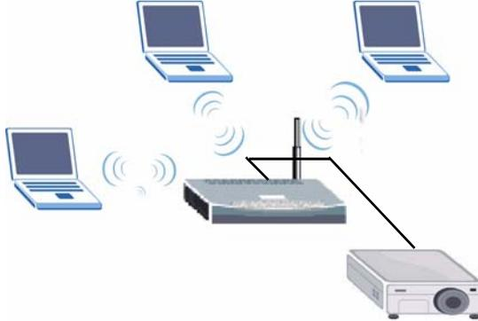
This Quick Start Guide shows how to connect to the WPA-1000 with an Ethernet cable in order to set it up and secure the wireless connection. (If the wireless connection is not secure, people in adjacent rooms may be able to view your presentation.) It also shows how meeting participants can connect wirelessly to the WPA-1000 and use the WPA-1000 to display their presentation.
