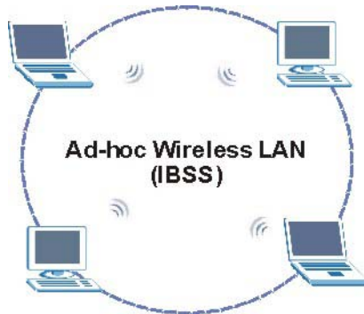
Diagram D-1 Peer-to-Peer Communication in an Ad-hoc Network
