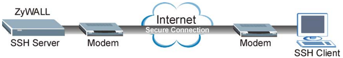
Figure 17-11 SSH Communication Example
