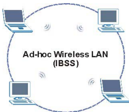
Diagram E-1 Peer-to-Peer Communication in an Ad-hoc Network
